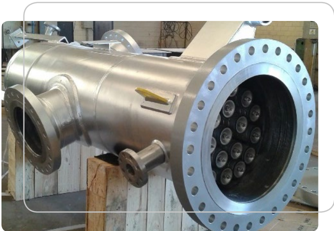
Oil & Gas - Compressed Air Filter Coalescing (Platforms P74 and P76)
