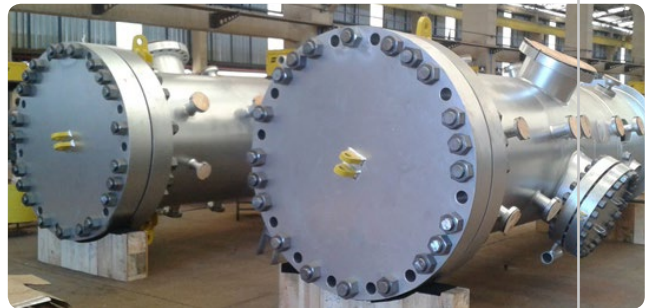
Oil & Gas - Compressed Air Filter Coalescing (Platforms P74 and P76)
